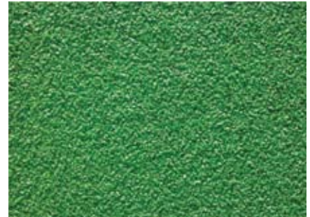
Tufted synthetic turf, generally sand-filled
