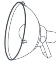
Type A floodlight giving a symmetrical beam
