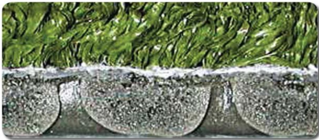
1st Generation Artificial Grass © Loughborough University; www.sportsurf.lboro.ac.uk • 10 – 12 mm fibre length, integral shock pad developed 1960s, nylon, unfilled, hard, abrasive • Used for hockey at the 1976 Montreal Olympics
