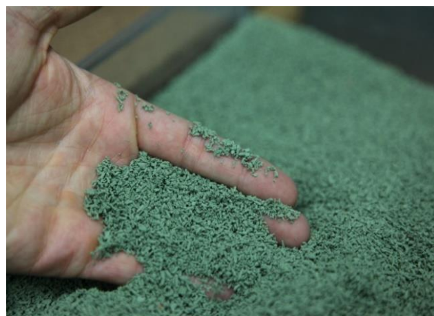
Photo 18: EPDM infill (source: Smart Connection Consultancy)
