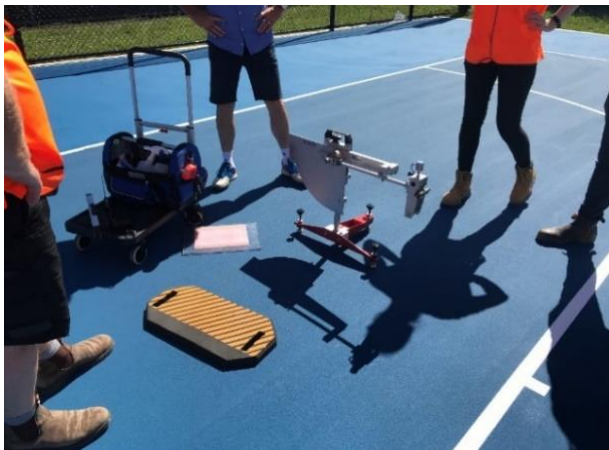
Photo 26: Testing apparatus for slip resistance
