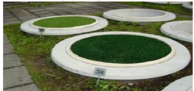
Photo 32: Swiss Study collecting rainwater through various synthetic sports surface systems
