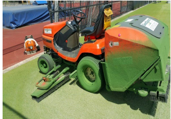
Photo17: The yarn has been exposed to UV and the tips are breaking down and covering the maintenance machine
