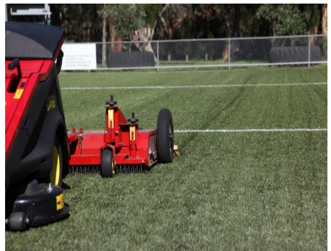
Photo 10: Tines being used to decompact infill and redistribute infill
