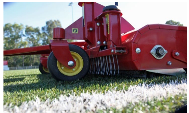
Photo 15: Modern machine providing height options for the tines to be used into the turf by an experienced operator
