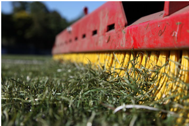
Photo 14: Brushes towed behind small tractor machine is better than a drag mat
