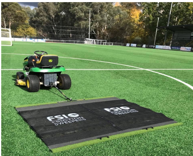
Photo 11: Friction Sweeper – Soft grass covered under-surface (source: Friction Sweepers International)
