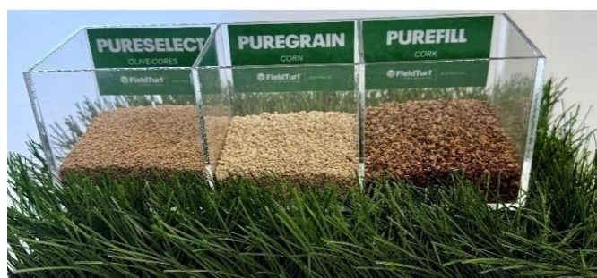
Photo 3.3: Organic infill options from one company, Fieldturf, other options include: woodchip, walnut husk, Pine chips and more. All reducing the UHI effect on local communities
