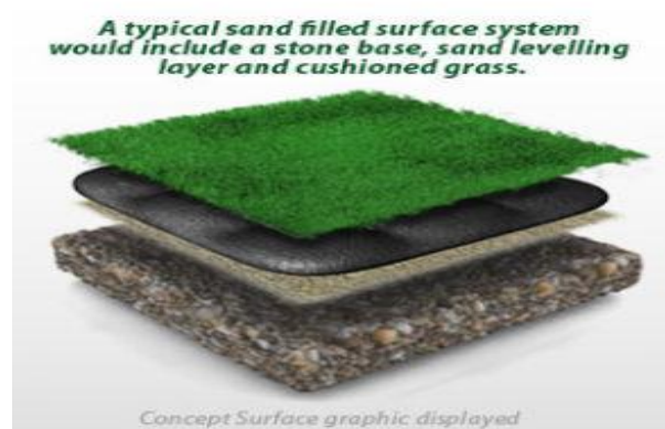
Figure 4.6: Sand Filled Carpet (source: ABS Sport Surfaces)
