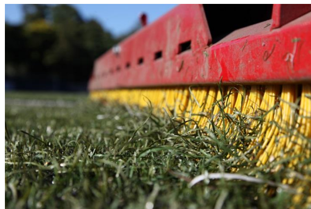
Photo 9.3: Brushes towed behind a small tractor machine is better than a drag mat
