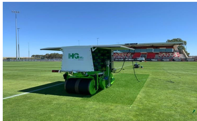
Photo 2.18: Desso GrassMaster System which is the first global 'stitch I' system, mainly used for stadium but now a more portable unit can be used for local government fields
