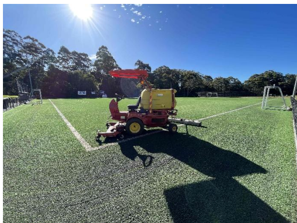
Photo 9.7: Machinery, including the metal magnet at rear (Source: Sports Clean)
