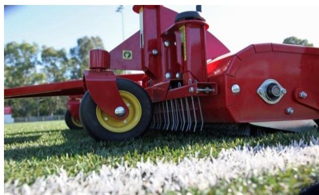
Photo 9.4: Modern machine providing height options for the tines to be used into the turf by an experienced operator
