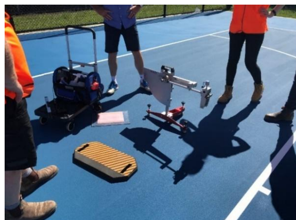
Photo 2.10: Testing apparatus for slip resistance
