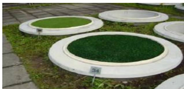
Photo 3.5: Swiss Study collecting rainwater through various synthetic sports surface systems
