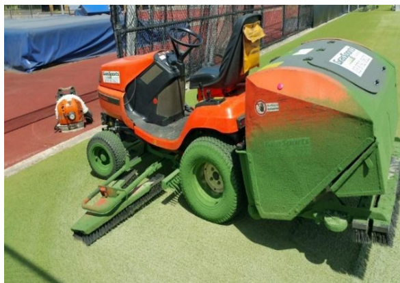
Photo 9.6: The yarn has been exposed to UV and the tips are breaking down and covering the maintenance machine
